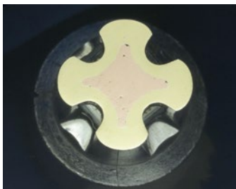
Figure V-1: Cross-section of a flawless sample
