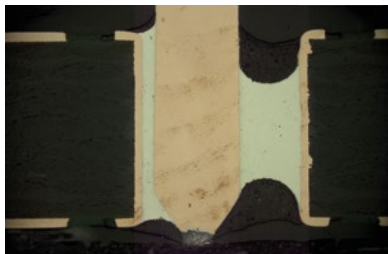
Figure VIII-11: Soldered joint with borderline degree of filling
